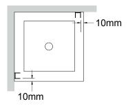
Wall retainers positioned 10mm in from edge of tray.
