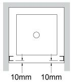
Wall retainers positioned 10mm in from edge of tray.
